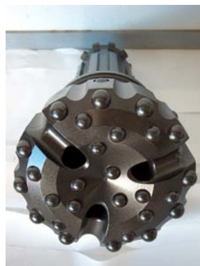
Fig. 2 -- Diamond Enhanced Hammer Bit
