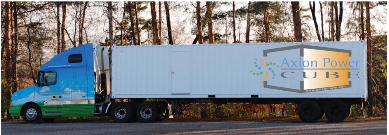
The Power Cubeis being commissioned onsite at Axion's plant. It can be configured to provide 1MW of power with fast discharge (responding in milliseconds) and fast full recharge (less than 10 minutes).
